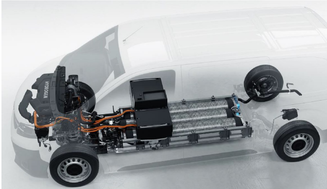
Figure 3 - Hydrogen Light Commercial Vehicle architecture
