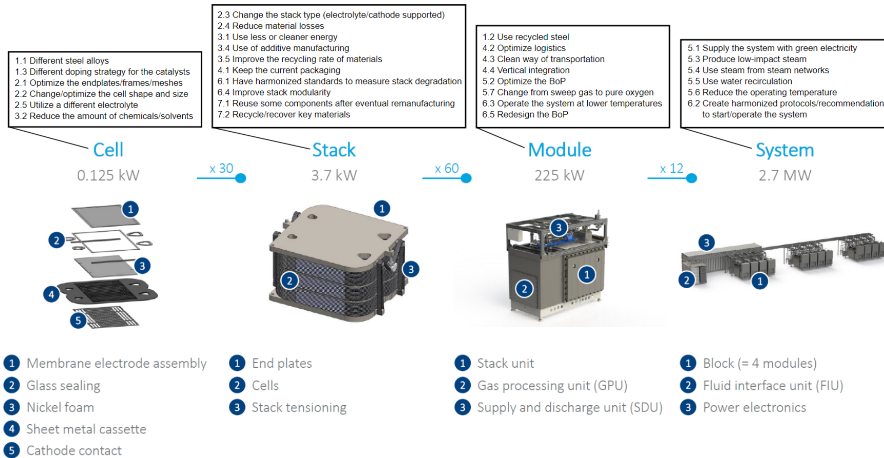
Figure 3. Schematic of the solid oxide system and eco-design actions in developing product concepts. Original image courtesy of Sunfire GmbH
